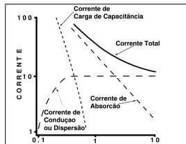
1. Capacitance charging current. This current is initially high and drops as the insulation becomes charged up to the applied voltage.
