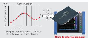
Maximum time to record to the internal storage memory (Abridged) \* The maximum number of channels to be used is 16 because memory for recording to the internal memory is allocated to each input unit.
