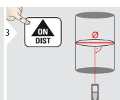
Aim laser perpendicular to the middle of the round object.
