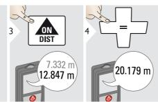
This process can be repeated as required. The same process can be used for adding or subtracting areas or volumes.
