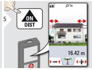
Select arrows with the cursor keys or by tapping on the display and adjust with softkeys. Corresponding width is calculated.
