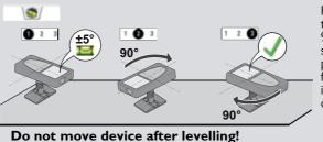
Rotate the device two times clockwise 90°. Follow the instructions on the display. Levelling is finished when OK icon appears on the display.
