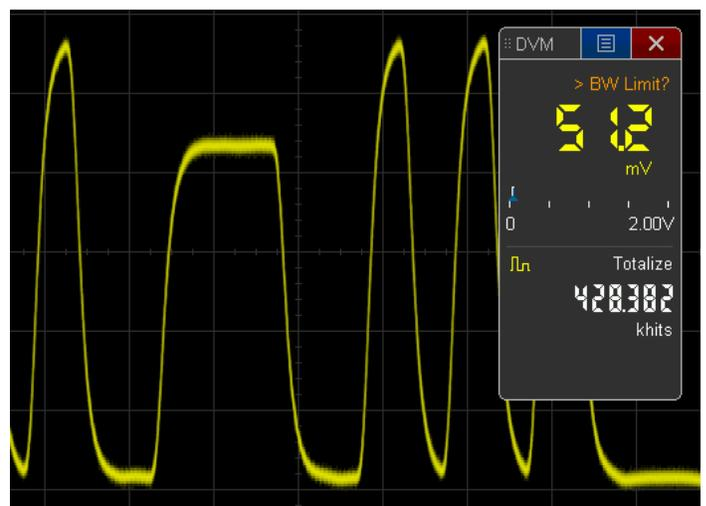
Figure 35. Totalizing the number of runt errors.
