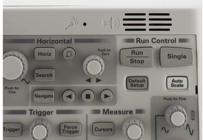
Figure 39. Voice control microphone and speaker.
