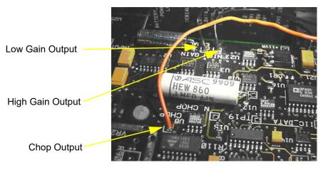
Figure A-10 Different view of the modified Measurement PCB
