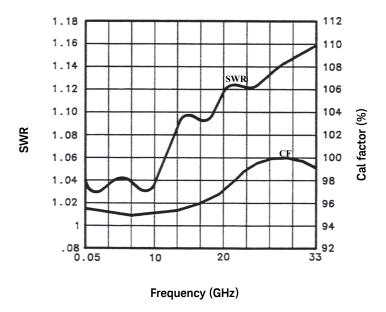
Figure 1-6 Typical CAL FACTOR and SWR vs. Frequency
