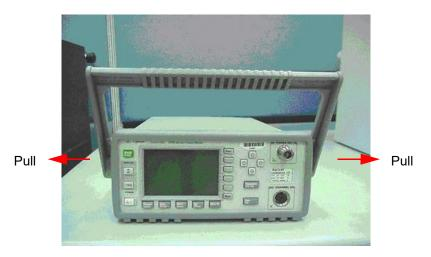
Figure A-2 Remove the power meter handle
