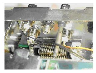
8 Securely fit the three BNC connectors into the three holes in the rear panel, as shown in Figure A-8. Use the 25 lb/in torque wrench to tighten the nuts.
