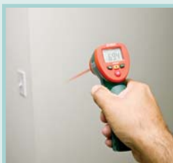
Check building for insufficient insulation
