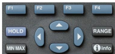
4. This starts the recording process. The Min Max symbol will appear.
