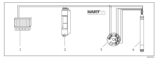
1 HART master, e.g. PLC (programmable logic controller)
