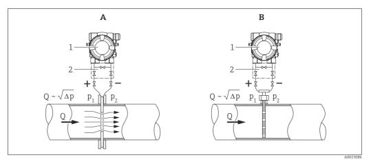
Flow measurement with Deltabar M PMD55 and Deltatop primary element
