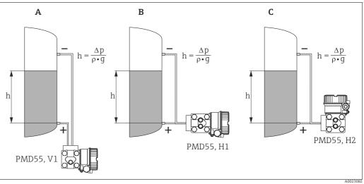
Level measurement with Deltabar M
