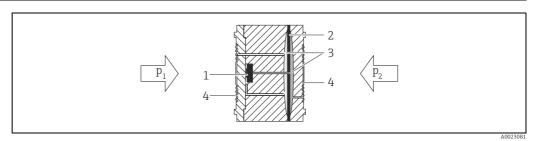
Measuring cell of the Deltabar M
