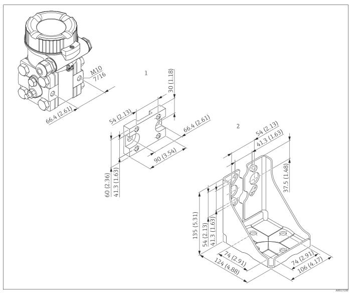
Mounting bracket for wall and pipe mounting
