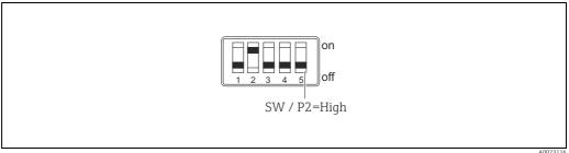
DIP switches in the connection compartment of the device. DIP switch 5 defines the high pressure side.
