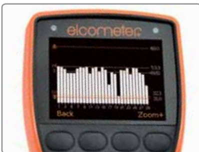
Individual batch readings can be reviewed numerically or graphically
