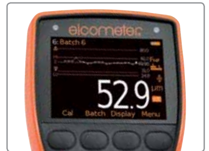
On-screen trend graph displaying last 20 measurement values
