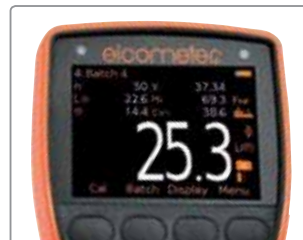
The gauge updates and displays the statistical values as each individual reading is taken
