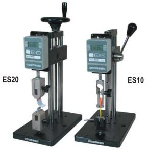
The ES20 is shown in a peel testing application with Series MG digital force gauge, and film & paper
