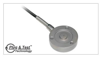
Series R02 button type smart sensors are designed for compression measurement applications in virtually every industry. Compact and rugged, Series R02 sensors are ideal for heavy duty applications with space constraints. Capacities available from 100 to 10,000 lbF [500 N to 50 kN]. Compatible with Mark-10 indicators (sold separately) through unique Plug & Test™ technology.
