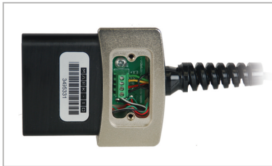
^ Cover is removed to expose the PCB with labelled wire connections and screw terminal block.
