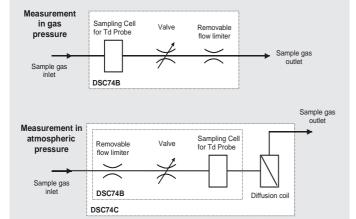
The DSC74B sampling cell enables the measurement of the sampled gas either in gas pressure up to 10 bar or in atmospheric pressure depending on the gas inlet and outlet. The DSC74C is like the DSC74B but with an additional coil to avoid back diffusion, the effect of surrounding moisture, in dewpoint measurements in atmospheric pressure.
