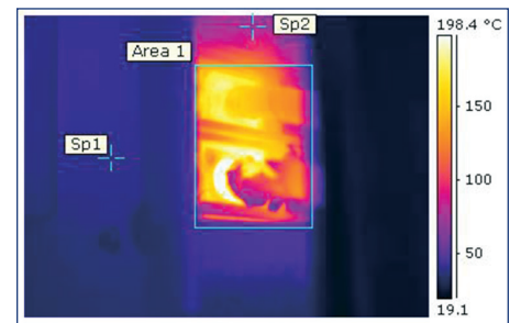
Figure 3. IR image showing a critical thermal fault on an electrical conductor at a fruit processing plant.
