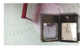
An experienced user may provide preliminary analysis on the chart output in the field, but communicating or storing the data electronically becomes possible only after a technician enters or scans the chart into a computer. This process can take days before results become available.
