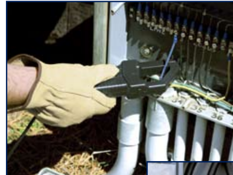
Model MD301 measuring AC current on a feeder.
