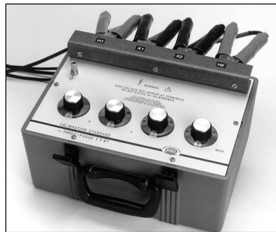
Calibration reference transformer
