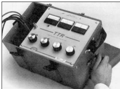
This single-phase TTR test set is operated by turning a crank.
