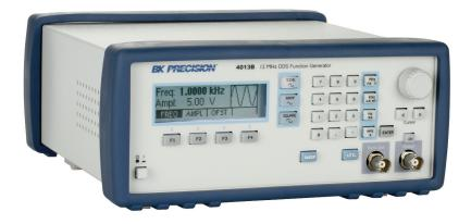
Models 4007B and 4013B are versatile DDS (direct digital synthesis) sweep function generators with high signal precision and stability. These instruments generate sine and square waveforms up to 7 MHz or 12 MHz, including triangle/ramp waveforms up to 1 MHz. Both models provide variable output voltages from 0 to 10 Vpp into 50 ohms or up to 20 Vpp into open circuit. A continuously variable DC offset allows the output to be injected directly into circuits at the correct bias level.
