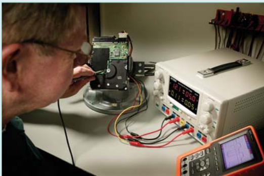
Single power supply with multiple DC outputs
