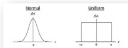
Figure 3: Measurement Uncertainty (Normal) and OEM Specifications (typically Uniform)
